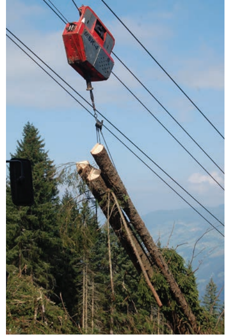
Above left: Glulam beam production at Jenbach Above right: Cable logging is used to harvest hard to access and steep forest
